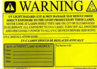
9: Warning Label (supplied) - Apply To: Access Doors/Ports/Panels
